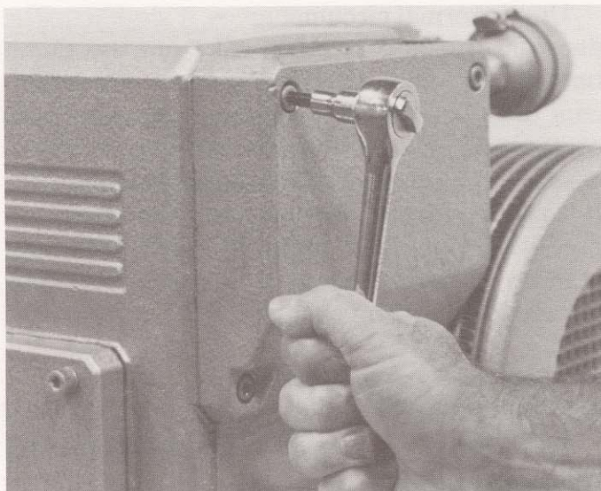
Figure 4 Removing Exhaust Housing
